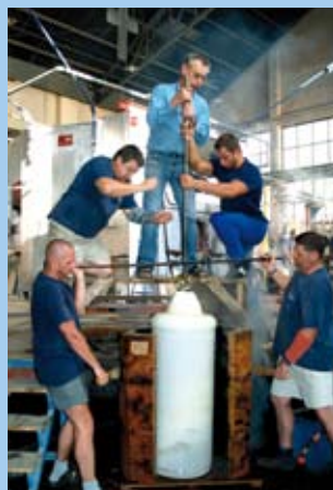
Production of an extraordinary mouth blown glass cylinder.
