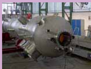
High pressure reactor in nickel base material, 37,800 kg. Hochdruckreaktor aus Nickelbasis- material, 37.800 kg.
