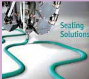
Foamed gasket with the MK 600 precision mixing head.
