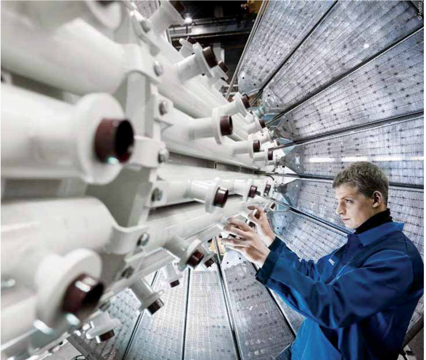
Specialists from the Andritz-Group - working on a filter shaft for a vacuum disc filter used in hard coal dressing.
